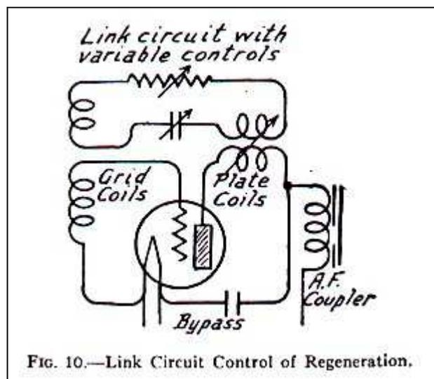
FIG. 10.—Link Circuit Control of Regeneration.
