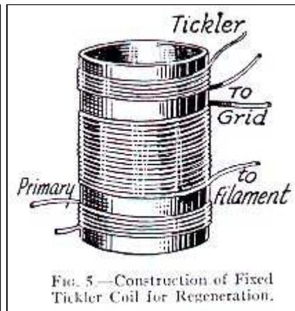
As the regeneration control condenser is tuned more and more closely to the frequency being received, the power absorbed from the grid circuit will increase and regeneration will be reduced.
