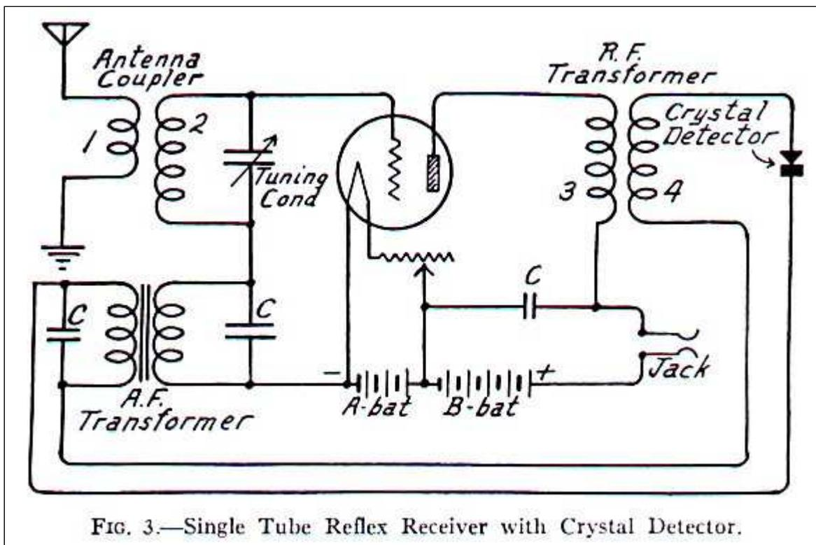
FIG. 3.—Single Tube Reflex Receiver with Crystal Detector.
