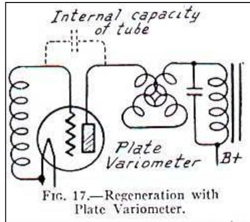
As the variometer's inductance is increased, the feedback through the tube capacity increases so that additional energy is sent back into the grid circuit. Reducing the variometer's inductance reduces the regeneration.
