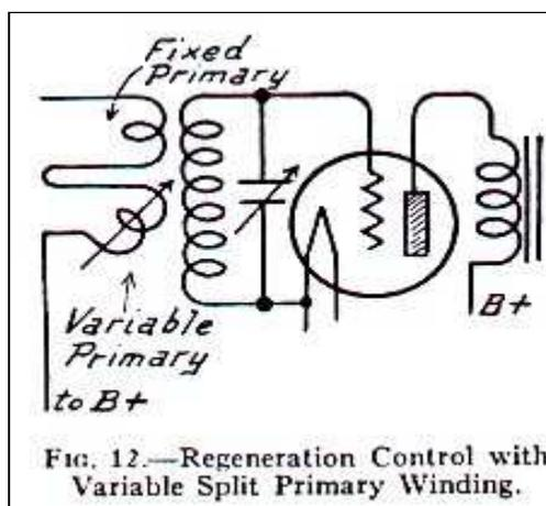
The split primary winding of [Fig. 12](#) has been used for automatic control of regeneration by attaching the movable part of the winding to the shaft of the tuning condenser. More regeneration is always required for low frequencies than for high frequencies, consequently the connection is made so that the two parts of the primary act together for maximum regeneration at low frequencies or high wavelengths.
