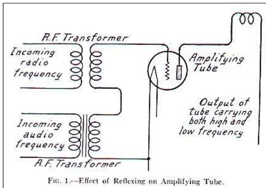
The high frequency output from the plate of the tube passes through the winding [3](#) which is coupled with winding [4](#) to make a transformer. The high frequency circuit is completed
