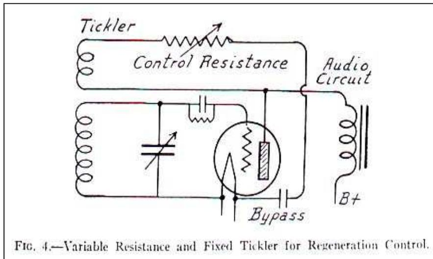
FIG. 4.—Variable Resistance and Fixed Tickler for Regeneration Control.
