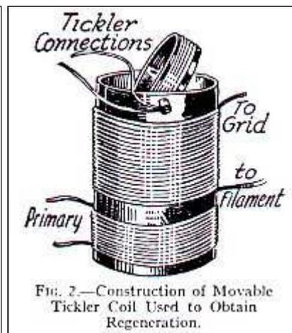
The connections are made exactly as shown in Fig. 7. The plate of the tube is connected to the tickler and the other side of the tickler is connected to the stator plates of the control condenser and to the primary of the audio transformer. The rotor of the condenser is connected to either filament terminal of the tube.
