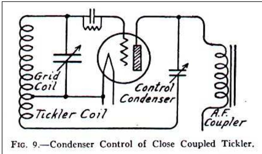
FIG. 9.—Condenser Control of Close Coupled Tickler.
