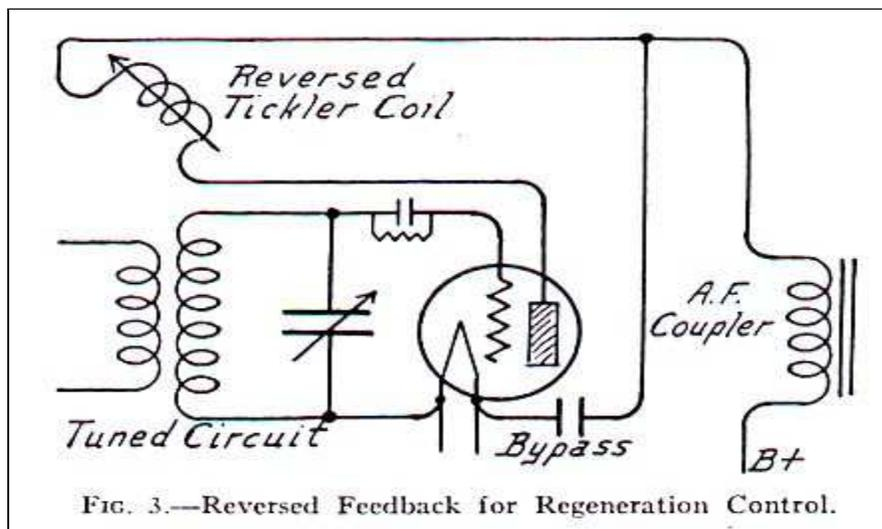
When the reversed tickler is in the position for maximum coupling, its feedback effect will be a minimum because it is opposing the voltages in the tuned coil. When the reversed tickler is at right angles to the fixed coil, regeneration will be maximum because then all of the opposing effect of the reversed tickler will have been removed.
