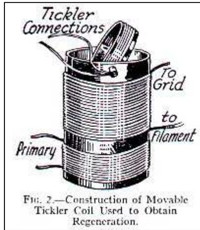
As the tickler is turned to increase its coupling to the stationary coil the effective inductance of the tuned stationary coil is increased. Therefore, the tuning point at which the circuit becomes resonant to a certain frequency will change with changes of tickler adjustment. This is a rather serious disadvantage of this method for obtaining regeneration since a receiver cannot be logged unless a note is made of the tickler coil setting.
