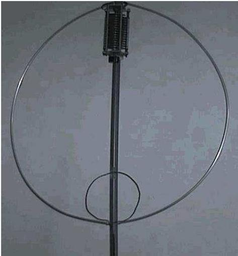
With these guides in place, I was able to create a former around which I could bend the aluminium rod to the correct shape.
