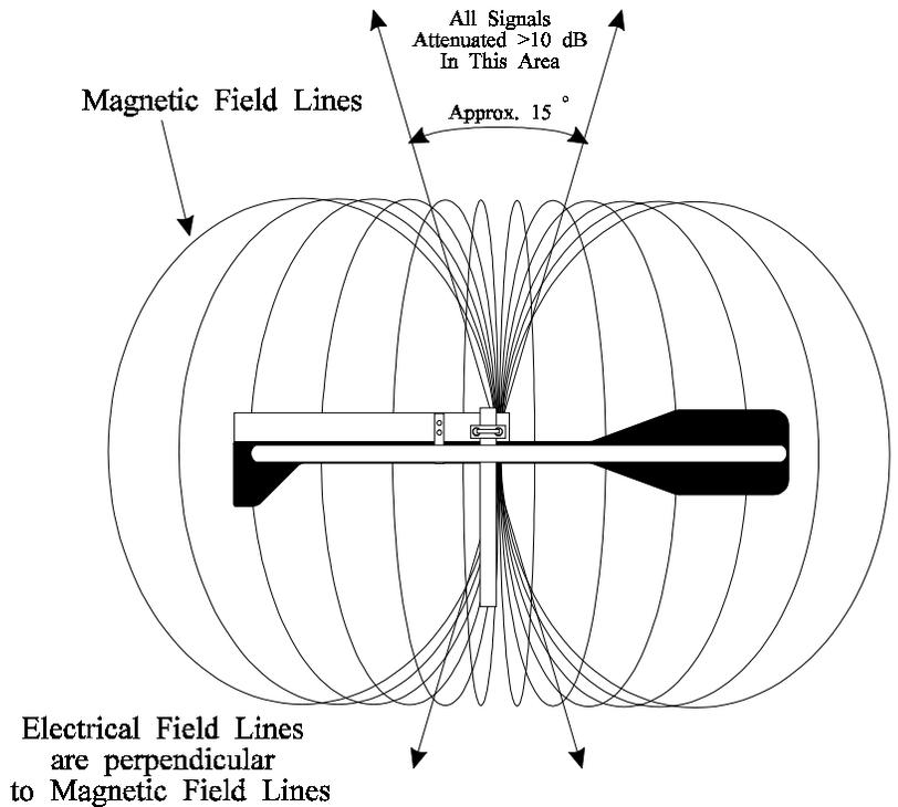
Electrical Field Lines are perpendicular to Magnetic Field Lines
