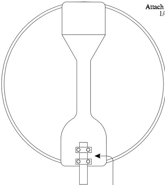
Each set of mast saddles is attached with one saddle plate and 2, 1/4-20, 2 1/2 inch long bolts
